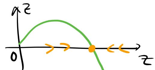
Sol'n:  $\frac{I(t)}{N} = \frac{dz}{dt} = \frac{1}{2} \left(1 - \frac{1}{r_0}\right)^2 \operatorname{sech}^2\left(\frac{r_0-1}{2}(t-t_0)\right)$
